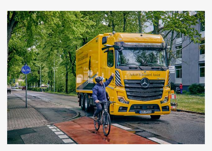
The Japanese Daimler truck subsidiary FUSO is also leading the way when it comes to safety: SGA which previously included a warning function but no braking feature, has been available for the Japanese market for all weight categories since 2020 – in the FUSO Canter, FUSO Fighter and FUSO Super Great. Since July 2021, the FUSO Super Great has also been offered with ADA 2 and the FUSO Fighter with ABA 5.
